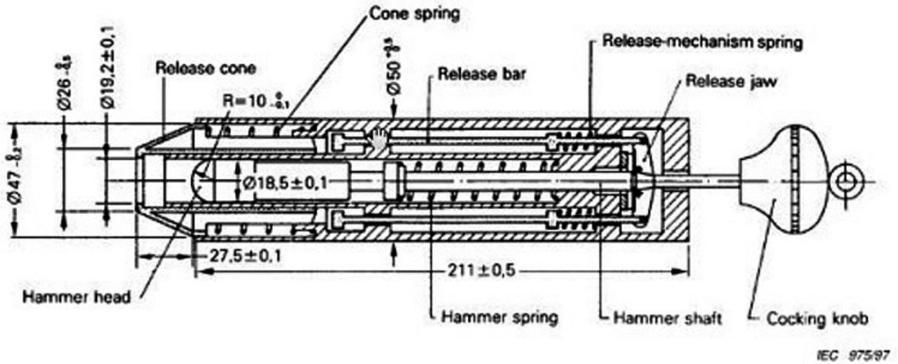
**Figure E.1 – Spring hammer test apparatus**
